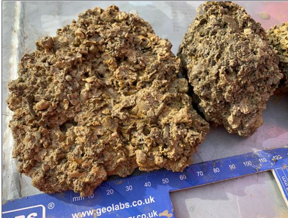
Plate 3.1 Coralline Crag sample recovered from approximately 17m depth in BH-RP-01
